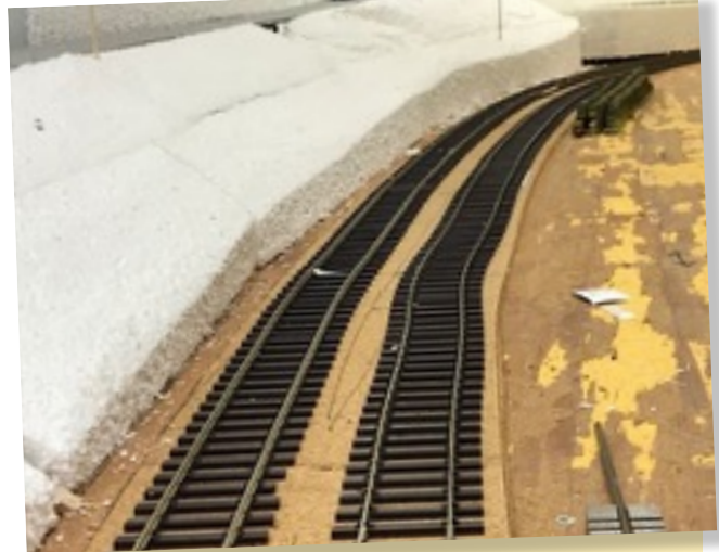
Distorted track following the hottest day of the year - although there is no thermometer in the barn the ambient temperature didn't seem to be all that high. I suspect the sun coming through the skylights in the roof void during the afternoon was the cause.
